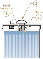
Maintain electrolyte level from at least 1/2-inch (13 mm) above plates to 1/4-inch (6 mm) below level indicator.
